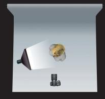
T: One D-lite RX4 head, one Clip-lock Stand, one Portalite Softbox Use the principles of 'Rembrandt' lighting to create the triangle of light on the face. Position the model's head at an angle and light it from the left side, so the side of the face closer to the camera falls into shade.
